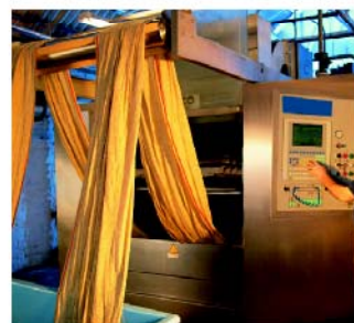
Fig. 9.10: Scouring by machines
