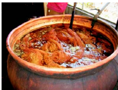
Fig. 9.9: Scouring in tanks
