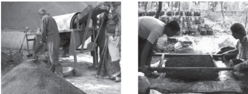
Fig. 5.4: Sieving Method: By Machine and Manual
