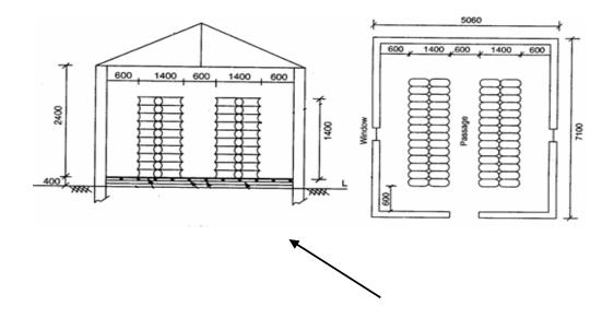
Fig. 8.1: A sketch of cement godown for stalking 500 bags of cement.
