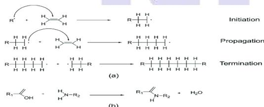
(b) **Condensation Polymerization:** In this, the monomers combine with the elimination of a small molecule like H<sub>2</sub>O, ROH or NH<sub>3</sub> etc. The reaction is called (step growth) condensation polymerization and the product formed is called condensation polymer.
