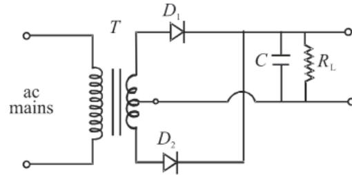
The capacitor C connected across the load to reduce fluctuations is called a filter capacitor.
