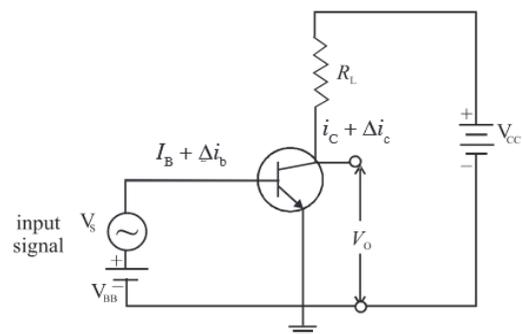
$$\text{Voltage gain, } A_v = \frac{V_o}{V_i}$$
