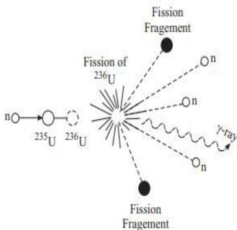
A substance like  ${}_{92}^{235}\text{U}$  which undergoes fission by thermal neutrons is called a fissile material
