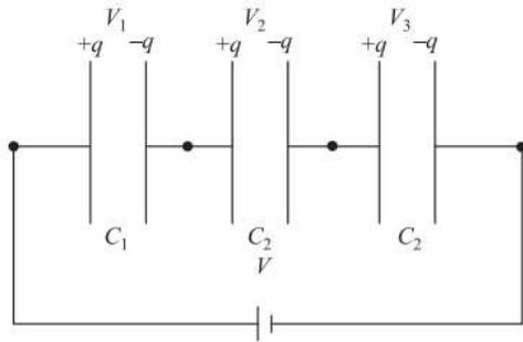
The second plate of the first capacitor is connected to the first plate of the second capacitor. The second plate of second capacitor is connected to first plate of the next capacitor of the combination and so on. The second plate of last capacitor of the combination is connected to the electrical source
