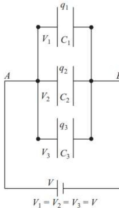
equivalent capacitance of a number of capacitors joined in parallel is equal to the sum of the individual capacitances. Remember that in parallel combination, all the capacitors have the same potential difference between their plates but charge is distributed in proportion to their capacitances
