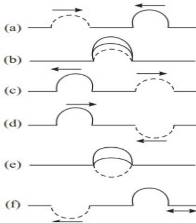
: At the points where the two pulses overlap, the resultant displacement is the vector sum of the displacements due to each of the two wave pulses. This is called the principle of superposition.
