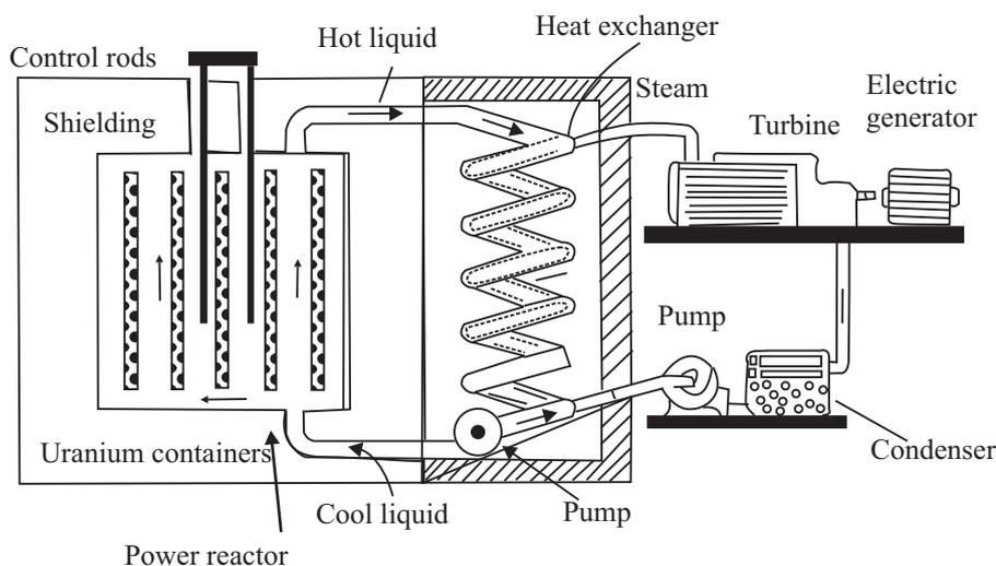
Fig. 27.5 : Schematic diagram of a nuclear reactor
