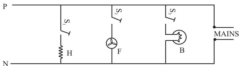
**Fig. 17.10 :** Arrangement of appliances in our homes. These are connected in parallel so that every appliance is connected to 220 V main supply. The total current drawn from the mains is the sum of the currents drawn by each appliance.
