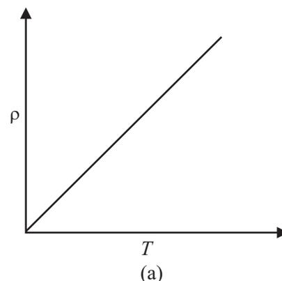
Fig. 17.14 : Typical resistivity–temperature graph for a metal
