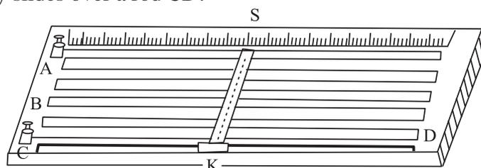
Fig. 17.21 : An illustrative diagram of a potentiometer
