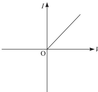
**Fig. 17.5 :**  $I-V$  graph for an ionic solution
