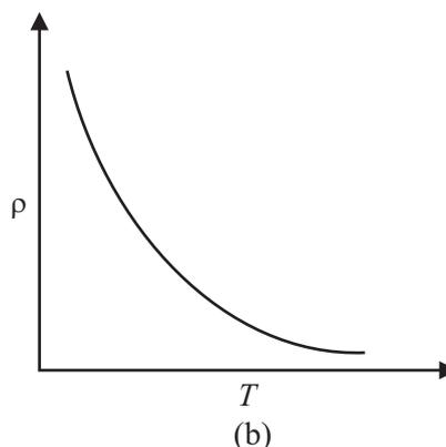
**Fig. 17.14(b) :** Resistivity of semiconductors decreases with temperature
