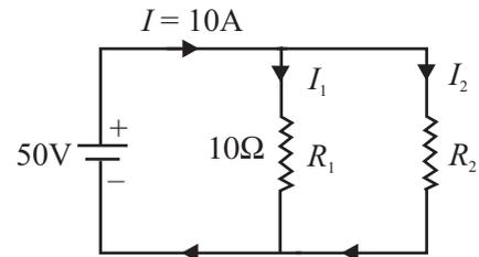
Fig. 17.11 : Two resistors in parallel
