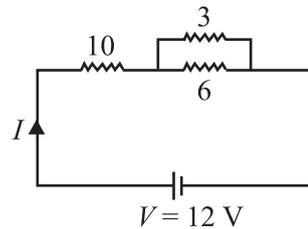
21. For the circuit shown here, calculate the value of current  $I$  and equivalent resistance  $R$ .
