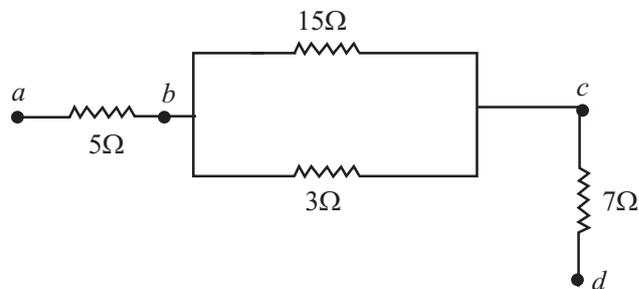
Fig. 17.12: A combination of series and parallel groupings
