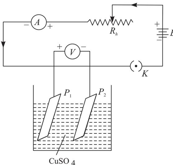
**Fig. 17.4 :** Electrical conduction through an electrolyte
