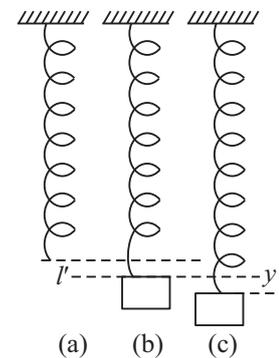
Fig. 13.6: Vertical oscillations of a spring–mass system
