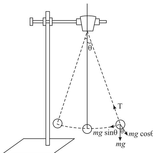
Fig.13.7 : Simple Pendulum
