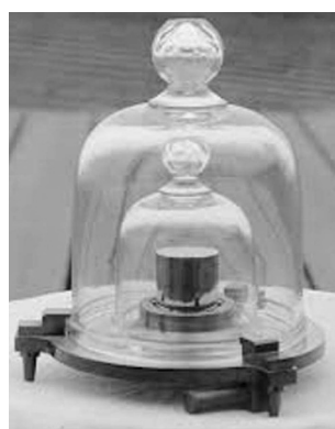
Fig. 1.1 : Prototype of kilogram
