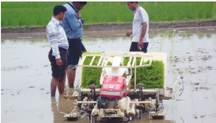
Fig. 6.11: Paddy transplanter for mechanical transplanting
