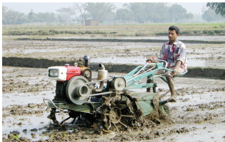
Fig. 6.8: Puddling of soil before rice transplanting in field
