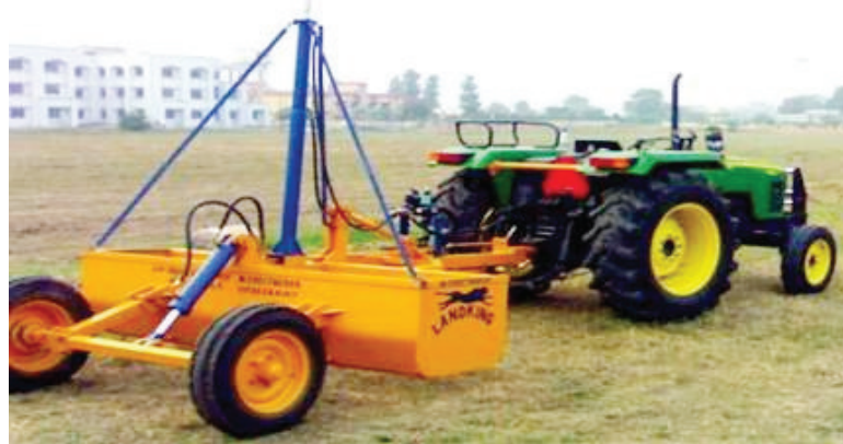
Fig. 4.2: Tractor-mounted laser land leveller
