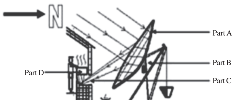
Fig. 31.6: Scheffler community cooker concentrator
