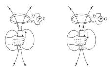
Current is induced only when the magnetic field due to the current in the circuit on the left changes.
