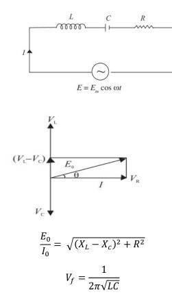
This frequency is called resonance frequency and at this frequency impedance is minimum.
