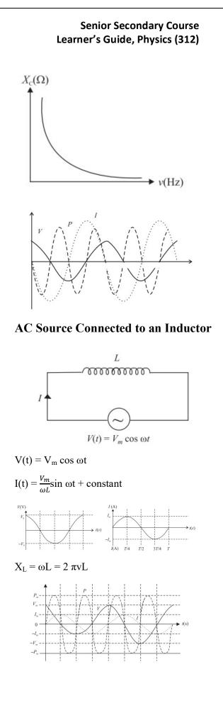
Inductive reactance is a measure of the extent to which the inductor limits ac current in the circuit. It depends on the inductance and the frequency of the generator
