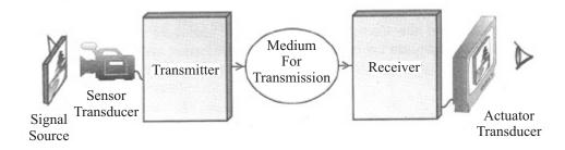
Fig. 30.1 : A schematic arrangement for the communication system.
