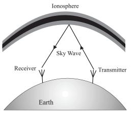
Fig. 30.9: Skywave propagation
