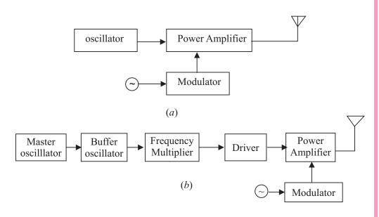
Fig. 30.13 Block diagram of (a) a basic and (b) practical AM transmitter
