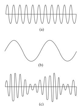
Fig. 30.12: Modulation of a carrier wave by a modulating signal: (a) a sinusoidal carrier wave of high frequency, (b) a modulating signal (message or information signal) of low frequency, (c) amplitude modulated carrier wave.
