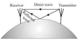
Fig. 30.10: Space-wave propagation
