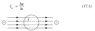
Fig. 17.1 : Motion of charges inside a conductor of surface area A
