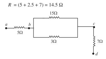
Fig. 17.12: A combination of series and parallel groupings
