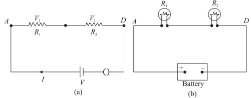
Fig. 17.8 : a) Two resistors connected in series to a battery, and b) two lamps joined in series connected to *a dc* source.
