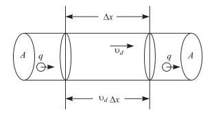
Fig. 17.2 : The charges move with a speed  $v_d$  through a surface of area A. The number of charges in a length  $\Delta x$  is  $nA v_d \Delta t$ .
