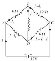
2. Examine the following circuit containing resistors and batteries. Calculate the current  $I_1$ ,  $I_2$  and  $I_3$ .
